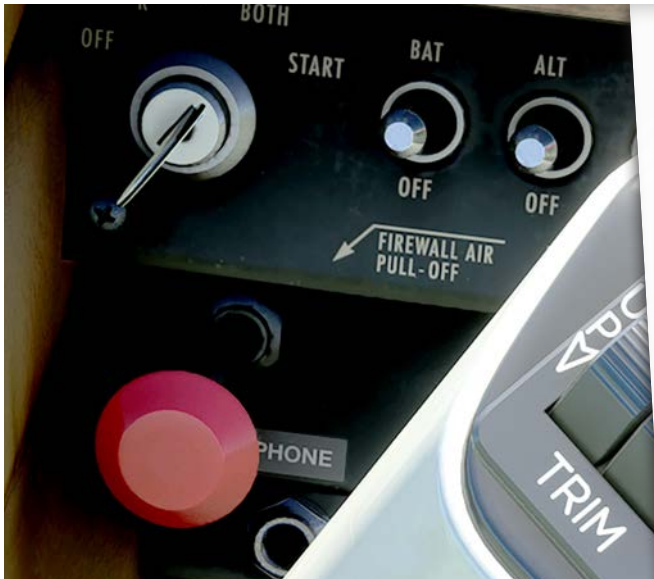
The V35 has a dedicated cutoff knob to prevent flames from following the heating system into the cabin. You must know the specific procedures and any special fire
