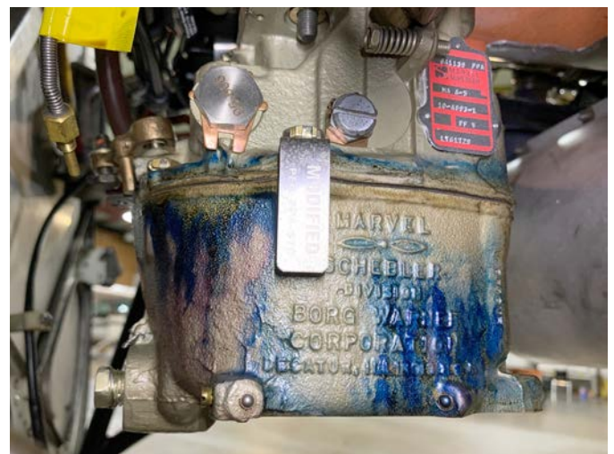
The best way to deal with fire is not having one in the first place. Chafed wires or fuel lines should be replaced immediately if discovered. Blue staining, as seen on this carburetor, indicates a fuel leak of 100LL and should be investigated. A dirty engine bay might not seem like a hazard, but excessive oil can accelerate deterioration of wiring and is a combustible material that's hard to extinguish.
